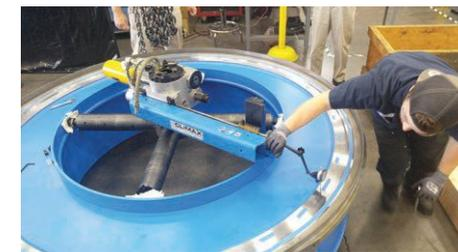
A portable flange facer being used to manufacture a circular mill.
