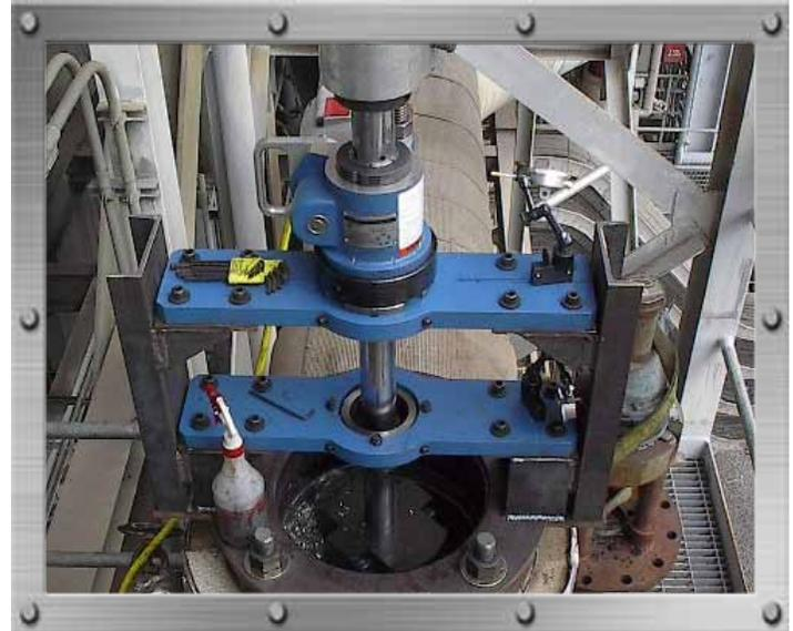
A Cantilever-Mounted BB5000 Boring
