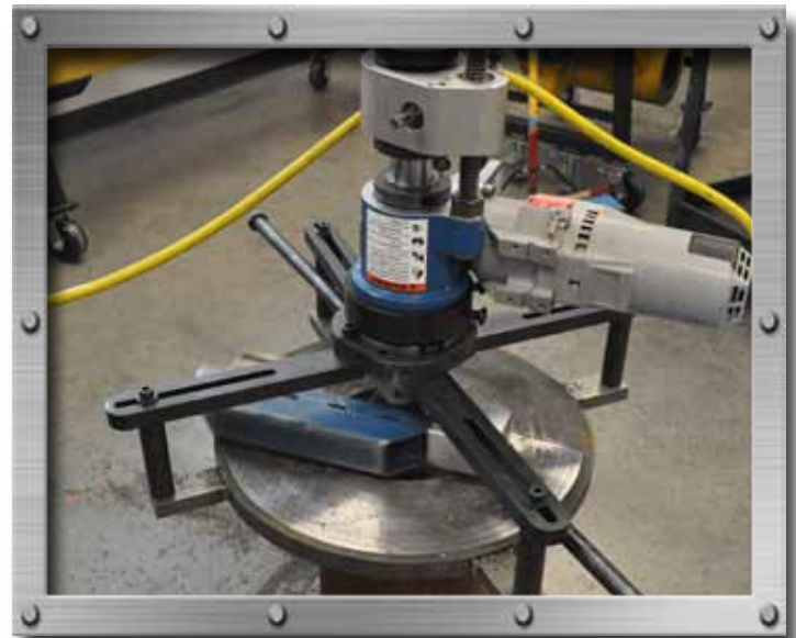
A BB5000 with a 12:1 RDU and extended universal leg mounts facing a large test part
